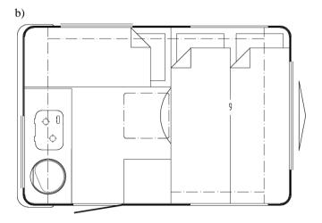
Fig. 4 Day layout (a) and night layout (b) of the N126nl caravan (1 - gas stove, 2 - sink, 3 - front sofa, 4 - long table, 5 - back sofa, 7 - hanging cupboards, 8 - side closet, 9 - sleeping spot of 130x193 cm).
