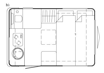
Fig. 2 Day layout (a) and night layout (b) of the N126nt caravan (1 - gas stove, 2. 2 - sink, 3 - front sofa, 4 - long table, 5 - bathroom, 6 - wardrobe, 7 - hanging cupboards, 8 - side closet, 9 - sleeping spot of 130x193 cm).
