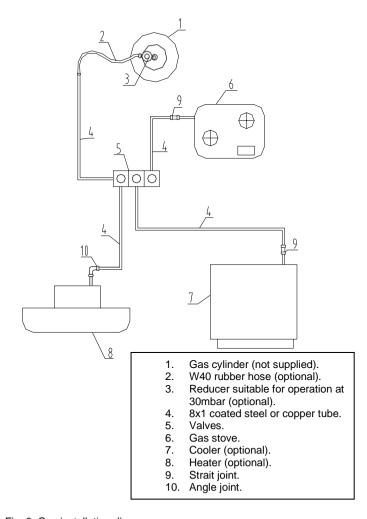
Fig. 8. Gas installation diagram.
