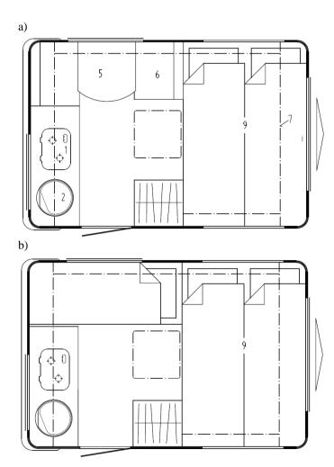
Fig. 3 Day layout (a) and night layout (b) of the N126nn caravan (1 - gas stove, 2 - sink, 5 - table, 6 - wardrobe, 7- hanging cupboards, 9 - sleeping spot of 130x193 cm).
